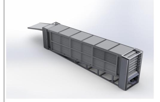
It cools the bread coming out of the oven and delivers it to the packaging area. Width 60 cm to ensure proper cooling of the product before packaging
